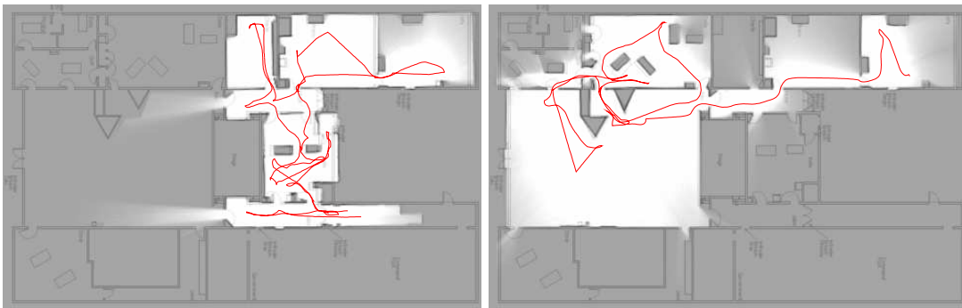
Fig. 10. Individual maps for two of the four robots, generated using the single-robot algorithm.
