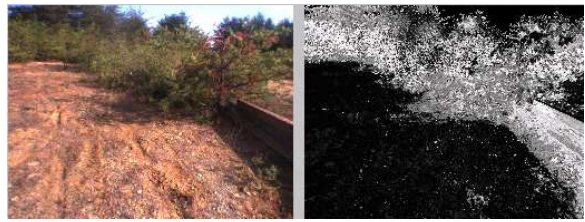
Fig. 6. Color-predicted cost in test 7 (Grayscale maps to cost)
