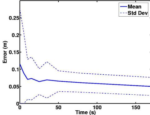
Fig. 9. The mean error between the robots' positions and the centroids of their Voronoi regions is shown as a function of time for an experiment with 20 robots. Because of sensor noise, we used a fixed error threshold of 0.075 m. Robots with desired positions within this distance remained stationary, limiting the convergence of the mean error.
