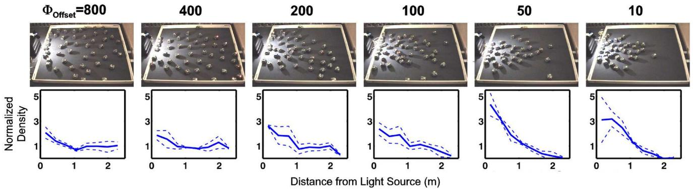
Fig. 7. The upper row of images show the final positions of 40 robots using the proposed control law. The sensor offset,  $\Phi$ , is labeled above each picture. The graph below each image plots the normalized density of the robots as a function of their radius from the light source. A uniform density would appear as a horizontal line with a value of one.
