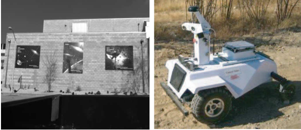
Fig. 8. Sample image (left) from experiments using a stereo setup configured analogously to the LAGR robot (right). The wall is approximately 20m from the robot. This sequence uses rectified camera models with a resolution of 512 \times 384 pixels, a horizontal FOV of 54.08^\circ , a vertical FOV of 40.87^\circ and baseline of \sim 18 cm.
