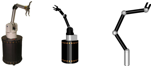
Fig. 2. Left: The UMass mobile manipulator with ten degrees of freedom. Middle: Model of the real platform. Right: Stationary robot with twelve degrees of freedom.
