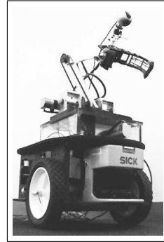
Figure 6. Our mobile manipulator with a two link arm and gripper.
