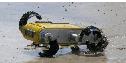
Fig. 11. The hexapod robot, shown equipped with semi-circle legs for land locomotion. The vehicle moves forward by constantly rotating legs in two groups of three, forming stable tripod configurations.
