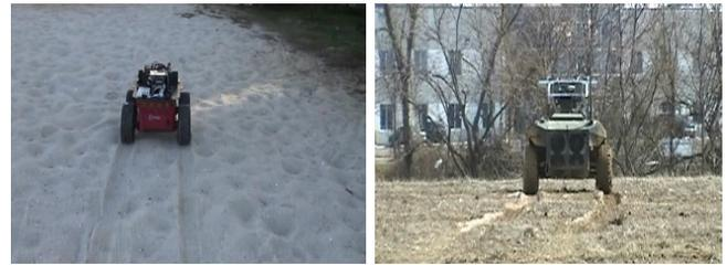
Fig. 2. (a) Pioneer 3-AT Robotic Platform on Sand. (b) XUV Robotic Platform on Mud
