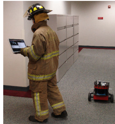
Fig. 1. Volunteer firefighter searching with a Pioneer mobile robot. The robot and humans execute a combined schedule that both clears the environment of an adversarial target and optimizes a non-adversarial target motion model. Our decentralized algorithm allows for robots and humans flexibly to fill the different search roles. The agents share their paths and an estimation of the target’s position.
