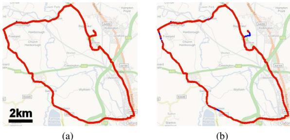
Figure 8: Loop closure maps for the 70km dataset. Sections of the trajectory where loop closures exist are shown in red. (a) The ground truth. (b) Detected loop closures using FAB-MAP (100k CL), at 100% precision. The recall rate is 48.4%. A total of 2,300 loop closures are detected, with no false positives.
