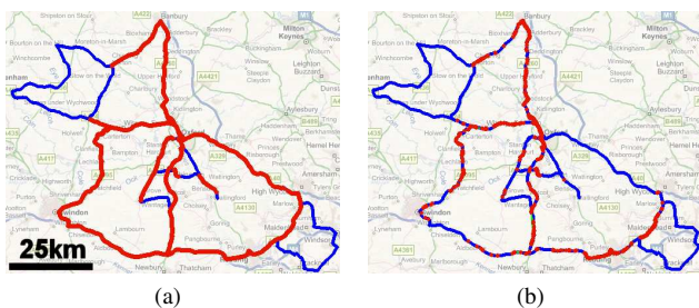
Figure 7: Loop closure maps for the 1,000 km data set. Sections of the trajectory where loop closures exist are shown in red. (a) The ground truth. (b) Loop closures detected by FAB-MAP (100k CL), showing 99.8% precision and 5.7% recall. There are 2,819 correct loop closures and six false positives. The long section on the right with no detected loop closures is a highway at dusk.
