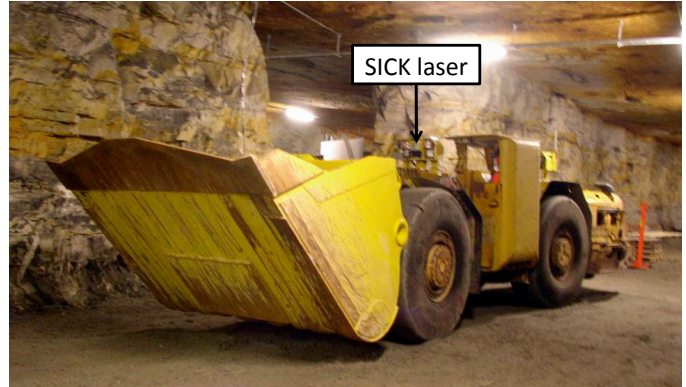
Fig. 1. Autonomous underground tramming vehicle used by Marshall et al. [14]; equipped with a SICK laser rangefinder and wheel/shaft encoders. We consider the same localization scenario as Marshall et al., which is a vehicle using a planar rangefinder to localize against a known map. As was the case for this system, we consider localization using the SPKF. Image credit: Atlas Copco.
