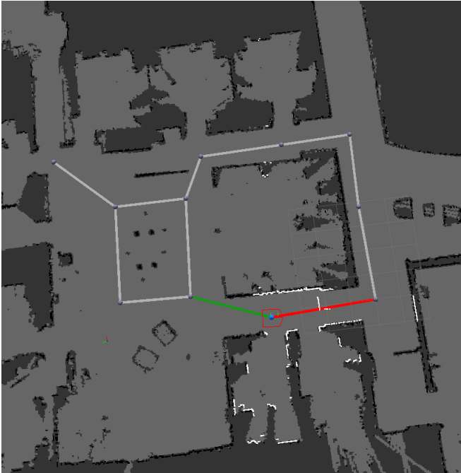
Fig. 8. Screenshot from visualization during execution on PR2 (on subset of overall environment used in experiments). The roadmap graph is overlaid on a static occupancy grid. The laser readings are also shown in white. The red polygon shows the robot’s current position, which is mapped to a particular node of the roadmap. An obstacle is visible in the hallway, resulting in the red edge being blocked. Thus the only available action is to follow the green edge. This figure is best viewed in color.
