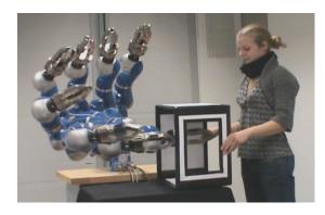
Fig. 1. KUKA LWR 4 robotic arm reaching through a hollow box with task being defined in combined Writhe and interaction mesh space, showing an example of planning and dynamic remapping using topological representations as described in Section V-B.
