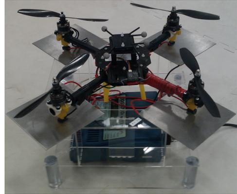
Fig. 3: Quadrotor docked at a charging station.
