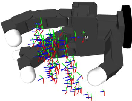
Fig. 5: Desired object centroid poses for all experiments. The colored, red, blue and green in each frame represent the x, y and z axes. The palm frame is represented by 'O' with arrows.
