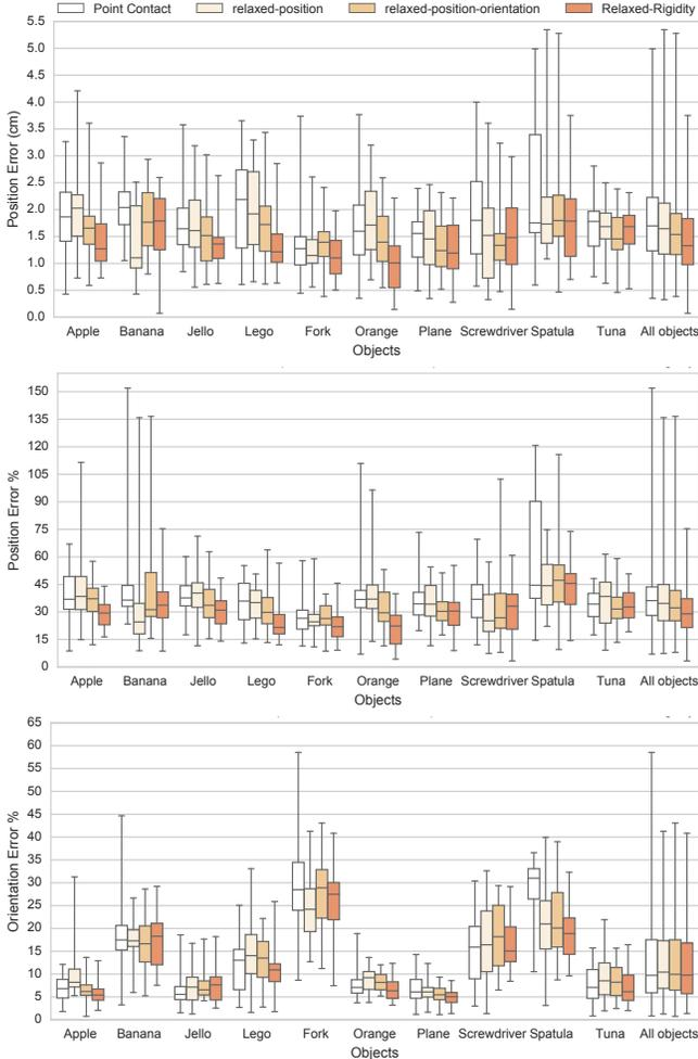
**Fig. 8:** A comparison of the relaxed-rigidity constraint performance with alternative formulations. Top: Position error Middle: Position error% Bottom: Orientation error%. The median position error decreases for all objects with our method. Except for *Banana* and *Jello*, the orientation error% improves for our method for all objects.
