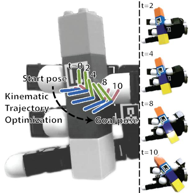
**Fig. 1:** Example trajectory produced by our method executed on the Allegro hand. The trajectory moves the Lego from its initially grasped pose to a desired pose. The robot follows the joint space trajectory produced from our trajectory optimizer with a PD based joint position controller. The images on the right show frames from execution where  $t$  refers to the timestep.
