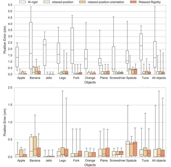
**Fig. 7:** Comparison of four different costs formulations for trajectory optimization: IK-rigid, relaxed-position, relaxed-position-orientation and Relaxed-Rigidity. Results show the position error between the desired final object pose and the final object pose obtained by the trajectory optimization. Bottom plot shows the same results without “IK-rigid” for improved reading.
