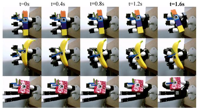
**Fig. 9:** Execution of in-grasp manipulation for four fingered and two fingered grasps. Frame “O” is the object pose and frame “G” is the goal pose. With the *Banana*, the ring finger loses contact during execution at  $t=0.4s$ , however the ring finger makes contact again at  $t=0.8s$  and the object reaches the desired pose. With the *Lego*, all fingertips maintain contact during execution.
