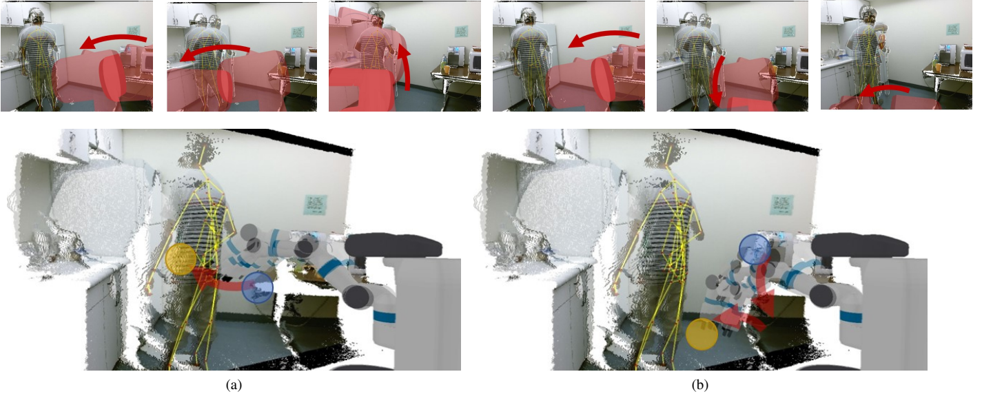
Fig. 4. Benefits of Occlusion-Aware Planning: The top row highlights the point cloud with the dynamic human obstacle, and the regions occluded by robot arms (in red). The bottom row highlights the trajectories computed by different planners when as the robot arm needs to move from right to left: (a) The trajectory is generated by the baseline planner, which does not account for occlusion. When the robot occludes the human, the motion prediction error is high and results in collisions. (b) The robot arm motion is generated by our occlusion-sensitive planner. The arm first moves to reduce the level of occlusion (i.e. a detour) and then reaches the goal to compute a safe trajectory.
