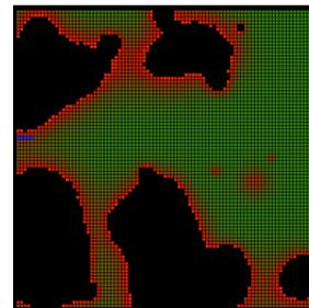
Fig. 3: Simulation environment, Weed World, created in Python. Each cell represents a small 0.8 m square portion of the field. The colors of the squares represent weed seed bank density. Darker colors represent higher density. The agents are shown in solid blue.
