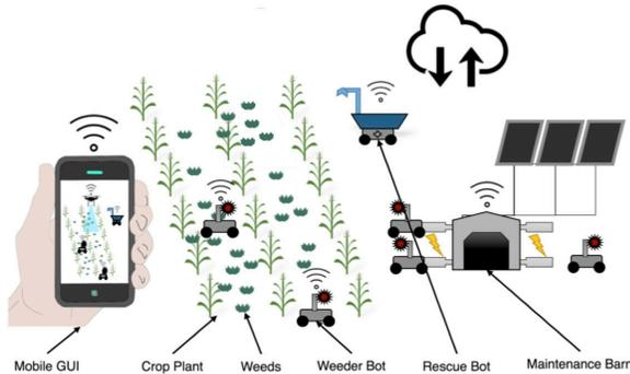
Fig. 1: The *agbot* solution for robotic mechanical weed control is a dynamically configured team of weeder bots, and automated maintenance barns for persistent autonomous weed control, leveraging collaboration.
