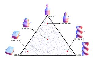
Fig. 1: Samples from a finite-dimensional subset of the Grasp Moduli Space spanned by the three surfaces displayed at the vertices of the triangle.
