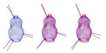
Fig. 8: Surface S with a stable grasp g (blue lines) and three deformations in the Grasp Moduli Space in a ball of radius 0.3, where only the contact and only the surface are deformed by a small amount in a) and b) respectively and where both are deformed in c). In all cases, the grasp remains stable after deformation.
