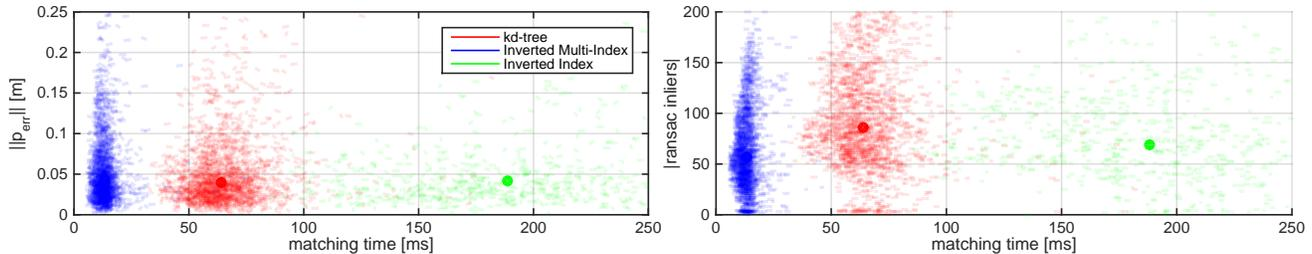
Fig. 3. Evaluation of different matching strategies: (Left) Position error of the global pose estimates computed from the 2D-3D matches established by each strategy. (Right) The number of inlier matches consistent with the estimated poses. The x-axis in both plots denotes the time required to compute the matches. Each point in the plots corresponds to a single pose estimate performed in the test sequence.
