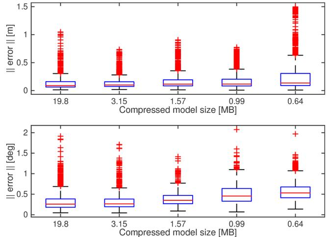
Fig. 2. Starting from an initial model of size 136.7 MB we apply a pruning technique to remove 3D points that have not been observed often. This reduces the model size to 19.8 MB. Combining pruning with a descriptor compression technique, we can fit the model in as little as 0.64 MB while not incurring substantial penalties on the localization quality. The plot shows the error statistics for (top) position and (bottom) orientation when localizing against models from different pruning levels.
