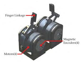
Fig. 5: Design of the two-finger parallel DDHand. The Motor drivers are not shown.
