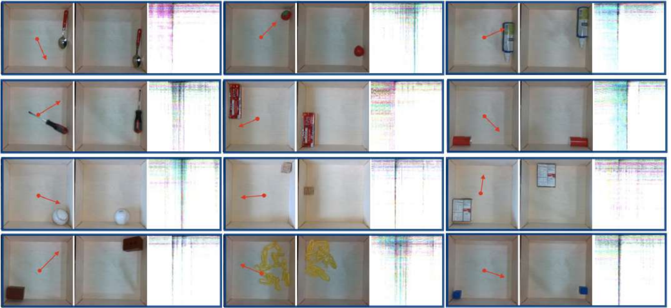
Fig. 3: Here are 12 interactions collected using Tilt-Bot. Each interaction is visualized as three images. The left image shows the visual observation of the object before the action is applied along with the applied action. The middle image shows the visual observation after the interaction, while the right image shows the STFT representation of audio generated by 3 of the 4 microphones.
