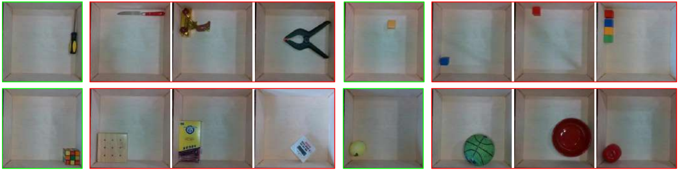
Fig. 9: Image retrieval results based on audio embedding. Here, the green box image corresponds to the query image and 3 images in the row (in red) correspond to the closest object retrievals in the audio-embedding space.
