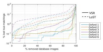
Fig. 5. Evaluation of recall integrity on the six OxfordRobotCar comparisons (the numbers correspond to appearance in table I). Lower is better.
