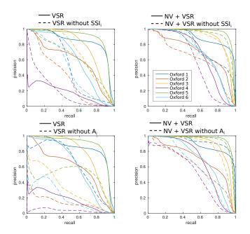
Fig. 6. Evaluation of the importance of  $SSI_i$  and  $A_i$  on the six OxfordRobotCar comparison. (*left column:*) Stand-alone VSR. (*right column:*) VSR in combination with NetVLAD. (*top row:*) VSR with and w/o  $SSI_i$  (using only  $A_i$ ). (*bottom row:*) VSR with and w/o  $A_i$  (using only  $SSI_i$ ).
