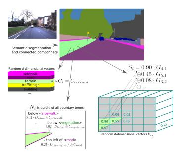
Fig. 3. Illustration of the spatial semantic information part of an image entity  $e_i$  consisting of class vector  $C_i$ , neighborhood encoding  $N_i$ , and shape/location encoding  $S_i$ . Together with the appearance encoding  $A_i$ , these vectors are the basis for the proposed vector semantic representation (VSR).
