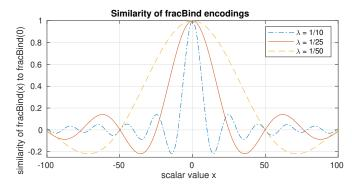
Fig. 2. Encoding similar scalar values with fractional binding results in high-dimensional vectors with high similarity. A scaling parameter  $\lambda$  can be used to influence the decay of the vector similarities. This resembles the sinc() function, the visible oscillation is a result of the periodic behavior of exponentiation in the complex domain, see [34] for more details.
