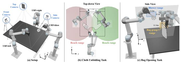
Fig. 2: System and Task Setup. Our system setup consists of (a) three UR5 robot arms, two of which are equipped with parallel-jaw grippers and one with a commodity centrifugal air pump. (b) shows a top-down view of the workspace and robots' reach range for the cloth unfolding task. (c) shows a side view of the workspace and the robots' action space for the bag opening task.
