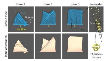
Fig. 3: **Simulating Air-Cloth Interactions.** Cloth is simulated as a spring-mass system, and airflow is simulated as a stream of invisible particles. Our policy only takes the color image rendered by OpenGL as input. This simulation environment is only used for training cloth unfolding task but not bag opening task.
