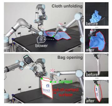
Fig. 1: **DextAIRity** manipulates deformable objects by controlling an active airflow. We demonstrate DextAIRity with two tasks that are particularly challenging for traditional contact-based manipulation: unfolding a large piece of cloth (top) and opening a soft bag and maintaining its opened state (bottom). By controlling the blower's direction, the system can apply dense forces on out-of-contact surfaces (A and B) to efficiently achieve its goal.
