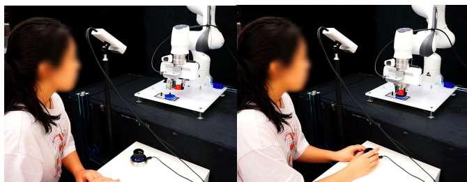
Fig. 10: Human Robot Teaming. Left: The robot executes the task by default while a human supervises the execution. Right: When the human detects undesirable robot behavior, the human intervenes.
