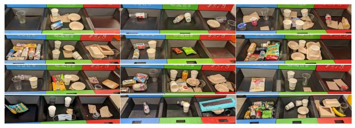
Fig. 4: Waste scenarios used for evaluations. Top 3 rows show the 9 in-distribution scenarios. The bottom row shows the held-out-scenes, containing objects previously seen neither in the real world nor in simulation, such as the keyboard, banana and face-mask.
