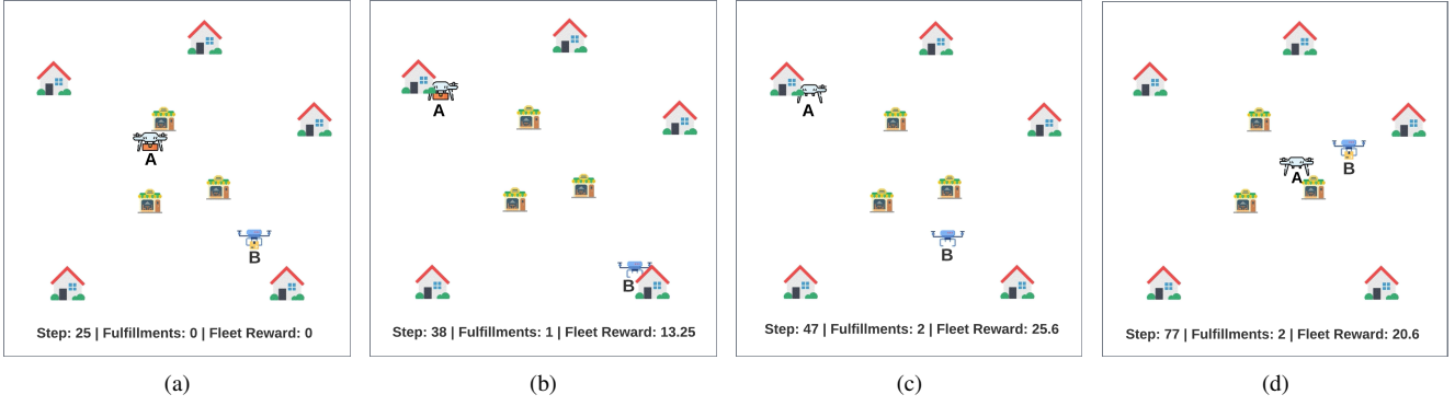
Fig. 6. Snapshots of a simple AAM simulation with 2 different vehicles, 5 clients, and 3 depots. (a) Both the vehicles are delivering payloads picked up at their initial depots to the clients. (b) An active timestep: B reaches the destination client, drops off the payload and collects a positive reward. A is still completing the delivery. (c) The next active timestep: A drops off the payload and collects a positive reward. B travels to a chosen depot to pick up another payload. (d) The next active timestep: A reaches an invalid depot, and collects a reward of -5 . B is on its way to deliver another payload. Elapsed \Delta t timesteps, total fulfillments, and the total fleet reward are displayed at the bottom of each image.
