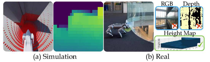
Fig. 5: Height map reconstruction from point cloud. (a) Go2 robot follows velocity commands while avoiding obstacles in simulation. Red dots show LiDAR points raycasting from the sensor center to the terrain mesh. The right image shows a preprocessed height map with values clipped to sensor constraints; darker colors indicate higher heights. (b) Safe locomotion near glass. The top-down height map detects glass surfaces where depth and RGB images fail.
