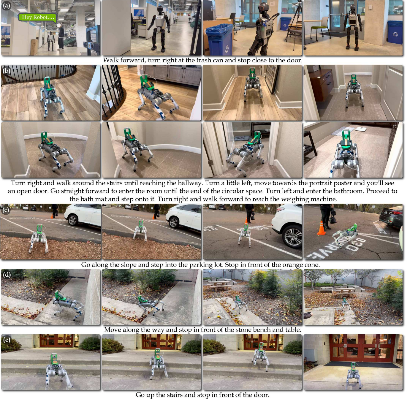
Fig. 7: Qualitative results from the real-world deployment of NaVILA. (a) We integrate speech recognition [70] into NaVILA, allowing a human to control the robot using voice commands that begin with "Hey Robot!". (b) The robot successfully handles long-horizon navigation tasks. Given a lengthy instruction, it moves through different areas of the house and stops at the specified goal. (c), (d), and (e) The robot demonstrates its ability to navigate through obstacles, traverse challenging terrains, and climb up and down stairs.
