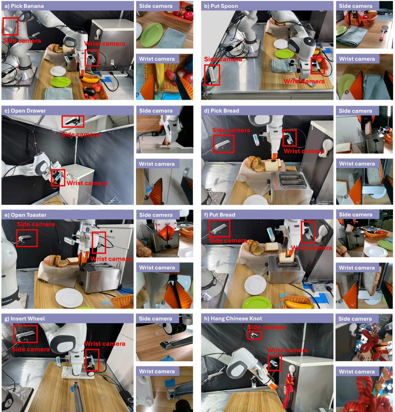
Fig. 5: Hardware setup and illustrations of camera views. We give the illustrations of hardware setup and the corresponding camera views for all real-world tasks in this paper, including a) Pick Banana, b) Put Spoon, c) Open Drawer, d) Pick Bread, e) Open Toaster, f) Put Bread, g) Insert Wheel, h) Hand Chinese Knot.
