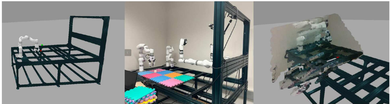
Fig. 41: Illustration of spatial alignment of simulation and real-world environments. Left: simulation environment, where robot control are tested, Middle: real-world teleoperation setup, Right: point cloud captured from the depth cameras accurately aligned with the virtual robot in the simulation, demonstrating a "digital twin" setup.
