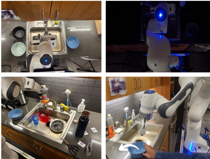
Fig. 10. Overview of the experiment setup for evaluating the robustness capacity of the generalist policy. upper left: multi-object scenario. upper right: dim lighting scenario. bottom left: messy kitchen scenario. bottom right: human disturbance scenario. See Table X for success rate.
