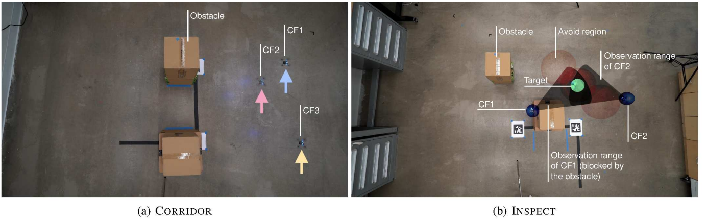
Fig. 8: Hardware tasks. We perform hardware experiments using a swarm of CF drones on the CORRIDOR and INSPECT tasks. In CORRIDOR, the team must cross a narrow corridor and cover a set of goals collectively without prior assignment. In INSPECT, the team must maintain visual contact with the target drone while staying out of the avoid zone around the target.
