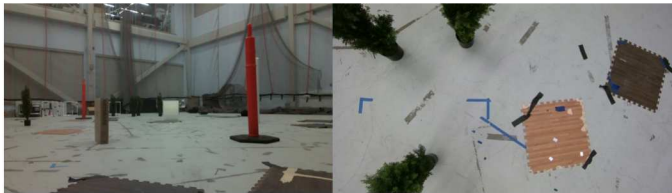
Fig. 5: Environmental setup used in the ground-aerial cross-view localization experiment as seen from both ground view (left) and aerial view (right).
