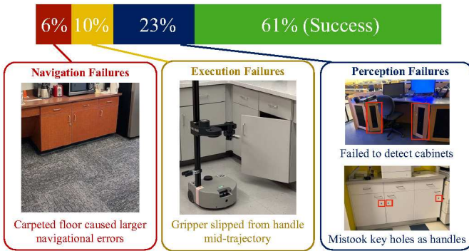
Fig. 8: Failure Cases. Bar chart characterizing the various failure modes of MOSART for opening drawers and cabinets. 59% of failures are due to perception failures, including failure to detect the cabinets outlined and confusing keyholes for handles. Other failures were during execution, where the handle would slip out, and during navigation, where navigating on carpets was less accurate than on tiles.
