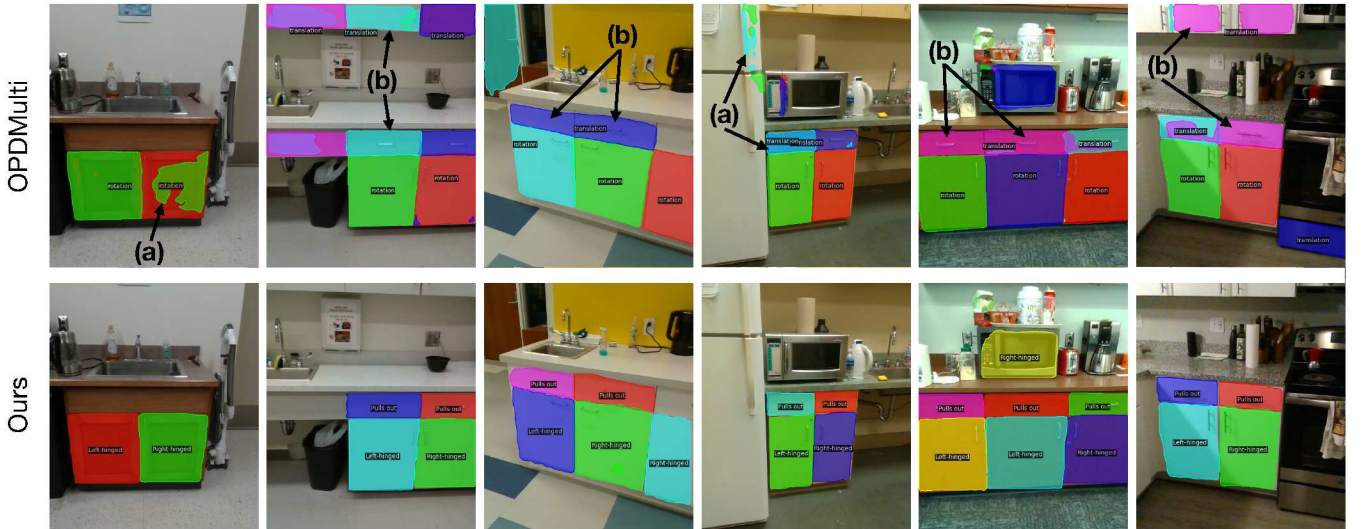
Fig. 6: Comparison to OPDMulti [76]. We perform a qualitative comparison to OPDMulti [76] (appeared in 3DV 2024) on the same six images presented in Figure A10. OPDMulti fails in various ways: a) segmentation masks bleed outside of the object, and b) merging of multiple objects into one. Our model produces more accurate segmentation masks (which affect the surface normal, and thus the navigation).
