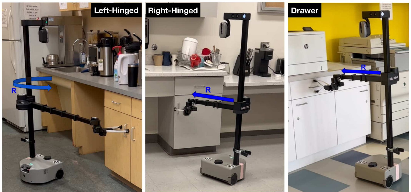
Fig. A11: Corrective Motions. We visualize the corrective motions for the different articulation types. For left-hinged cabinets, this is a counter-clockwise rotation in 1^\circ increments. For right-hinged cabinets and drawers, we extend the arm in 1\text{cm} increments. See Figure 4(a) and Section III.
