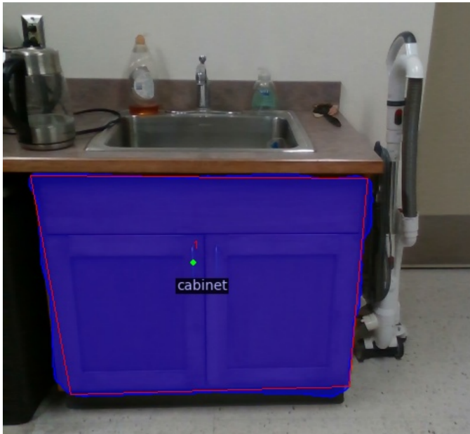
Fig. A13: Detic Failure. An example failure of using Detic to try and detect articulated objects. In this instance, Detic clumps multiple cabinets together
