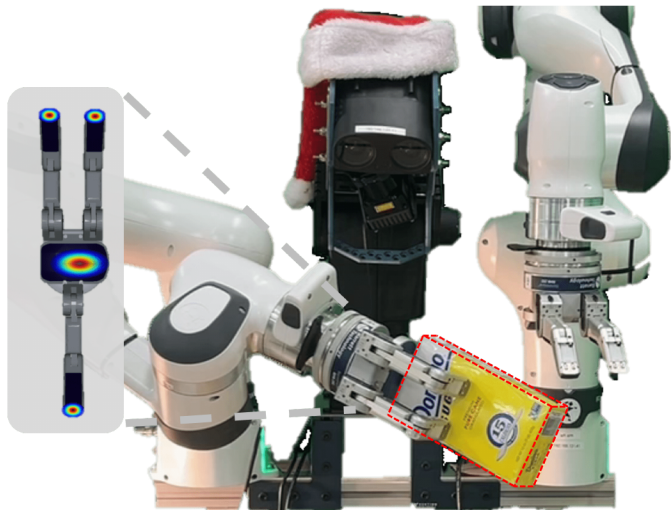
Fig. 1: Visuo-haptic sensing for 6D object pose tracking. We fuse egocentric visual and haptic sensing to achieve accurate real-time in-hand object tracking.
