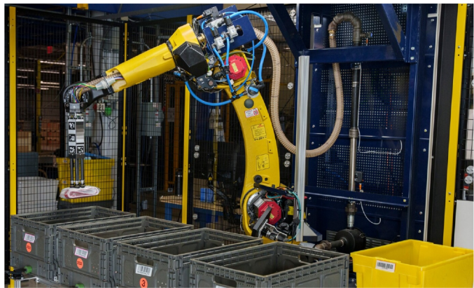
Fig. 1. Sparrow robot sorting products into bins in the Amazon warehouses.
