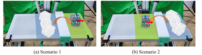
Fig. 11: (a) Scenario 1: The robot moves the object from the right to the left of the bump. (b) Scenario 2: The robot moves the object from the left to the right. The object’s initial pose is randomly set within the blue area. The robot must manipulate the object to match both the position and orientation of the goal pose sampled within the green area.
