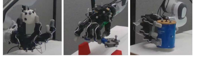
Fig. 10: Successfully grasping different objects using the proposed method
