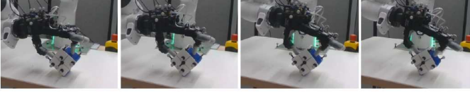
Fig. 14: Cube turning hardware experiment.
