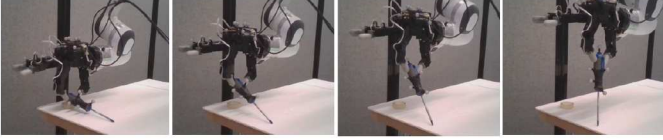
Fig. 15: Screwdriver turning hardware experiment.
