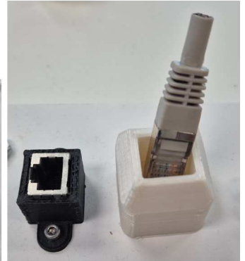
(h) Ethernet connector and socket. The connector is held in a custom holder.
