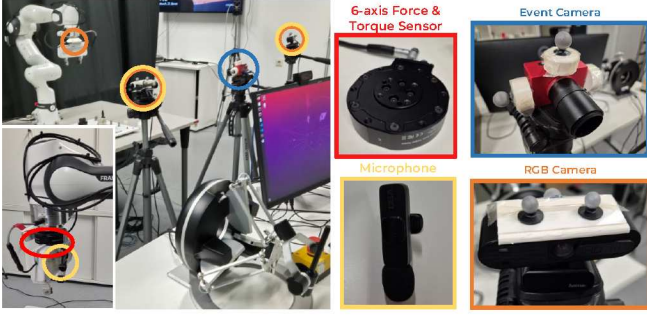
Fig. 2: Overview of the sensor placement. We use two external and one wrist-mounted RGB cameras (marked in orange). Additionally, we use an externally mounted event camera (in blue), three microphones (in yellow), and one wrist-mounted force/torque (F/T) sensor (in red). The omega.6 haptic teleoperation device is also visible.
