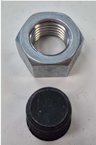
(e) Nut 4 and its socket. Approx. diameter: 25 mm.
