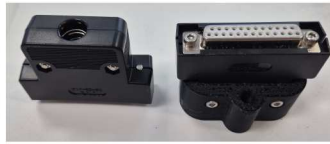
(b) D-SUB connector and socket. Approx. size: 60×20 mm.
