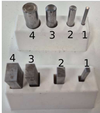
(f) Top: round pegs. Bottom: square pegs. Round peg diameters (sizes 1–4): 4 mm, 8 mm, 12 mm, 16 mm. Square peg dimensions (sizes 1–4): 4 mm, 8×7 mm, 12×8 mm, 16×10 mm.
