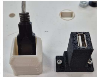
(g) USB connector and socket. The connector is held in a custom holder.
