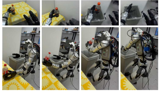
(b) Trash Bottle Throwing: The task begins with the robot stooping and turning its upper body to the left to grab the trash bottle. The robot then turns its waist about 90 degrees to the right and throws the trash bottle into the trash bin.
