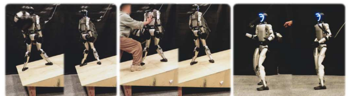
Fig. 11: Standing stability. Our control policies demonstrate great stability against external disturbances after successful standing up.
