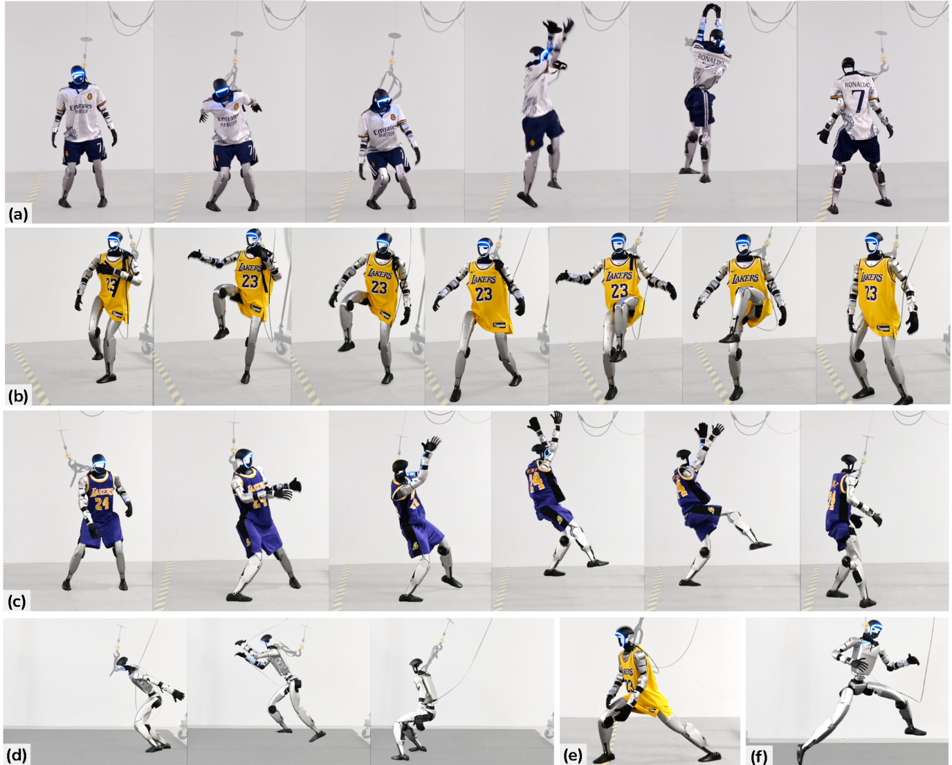
Fig. 1. The humanoid robot (Unitree G1) demonstrates diverse agile whole-body skills, showcasing the control policies’ agility: (a) Cristiano Ronaldo’s signature celebration involving a jump with a 180-degree mid-air rotation; (b) LeBron James’s “Silencer” celebration involving single-leg balancing; and (c) Kobe Bryant’s famous fadeaway jump shot involving single-leg jumping and landing; (d) 1.5m-forward jumping; (e) Leg stretching; (f) 1.3m-side jumping.
