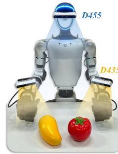
Fig. 14: Hardware Setup for Imitation Learning
