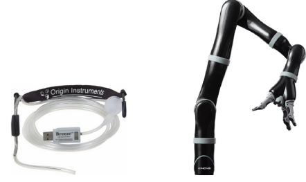
Fig. 4. Left: Sip/Puff Breeze USB interface with headset from Origin Instruments Corp. Right: Kinova Jaco 7-DoF robotic arm.
