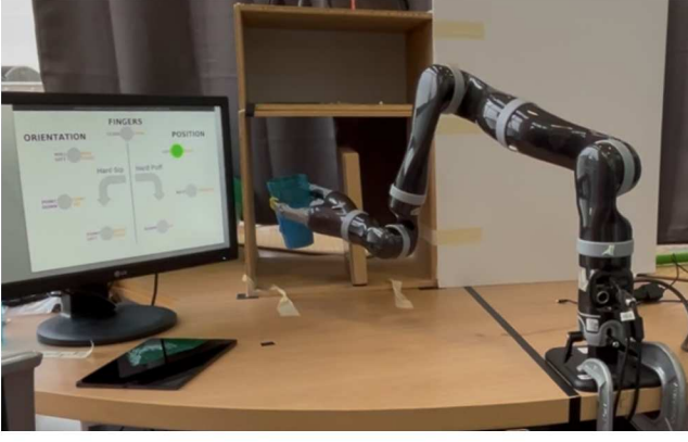
Fig. 6. ADL Task. The environment setup places a cup upside-down in the center of the upper shelf, and initializes the robot arm pose. The task proceeds as: (1) move the end-effector into the upper shelf, (2) grasp and lift the cup, (3) remove the cup from the upper shelf, (4) flip the cup right-side-up, (5) position the cup inside the left-hand compartment of the lower shelf, (6) open the gripper. A trial is considered successful if the cup is placed (gripper opened) in the target pose and orientation (inside lower shelf, right-side-up) within the time limit. A trial is considered unsuccessful if participants exceed the time limit, drop the cup, or do not achieve the goal pose and orientation.
