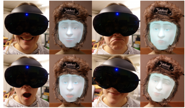
Fig. 1. An example of the Meta Quest Pro tracking the operator’s facial expression and displaying them on the Furhat robot in real-time.
