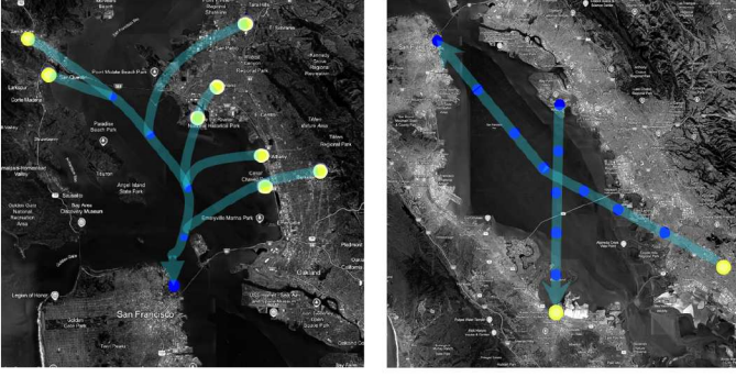
Fig. 6: Bay Area case scenarios. The left panel illustrates routes where multiple air taxi vehicles would travel from the North and East Bay toward San Francisco, merging into a single air corridor. The right panel shows intersecting air corridors: one where the vehicles would travel from Fremont (southeast) to San Francisco and another from Oakland (north-east) to Redwood City. The blue dots represent the waypoints that UAVs follow, while the yellow dots indicate the departure or an incoming waypoint of the corridor.
