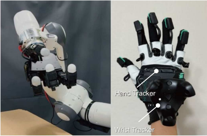
Fig. 6: Real world experimental setup based on Allegro Hand with a Franka Panda Arm (Left). We use human teleoperation (Right) as a proxy for high-level policy.
