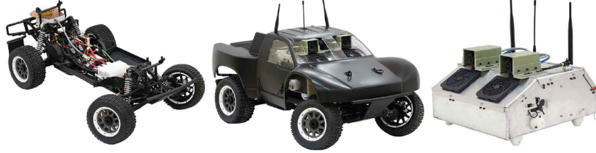
Fig. 17: AutoRally chassis and compute box [29].
