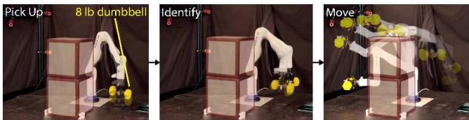
Fig. 4: An illustration of the third real-world experiment. The robot is required to pick up and perform system identification with an 8lb dumbbell and then follow a trajectory to avoid obstacles.
