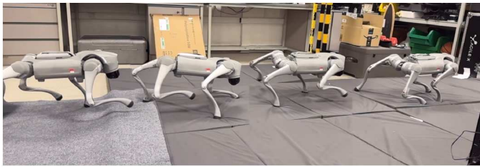
Fig. 12. Locomotion on 10cm thick soft mattress with a velocity command of 0.8m/s. Our robot stops with the right most posture when the velocity command is finally set to 0.
