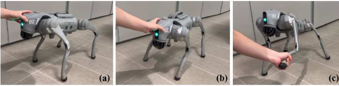
Fig. 6. Pushing the robot to its left (a) and right (b), and manually lifting its legs (c). In all those cases, the controller did not start trotting nor generate overreacting/hazardous motions.
