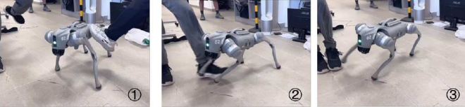
Fig. 7. Leg disturbance test with a) Backward sweep of the front legs, b) Backward sweep of the back legs, and c) Forward sweep of the front legs right after kicking its body. In a), the rear left leg also lifts up to help balance the whole body, while in b) the robot simply shifts its weight to the other three feet in response to the sweep.
