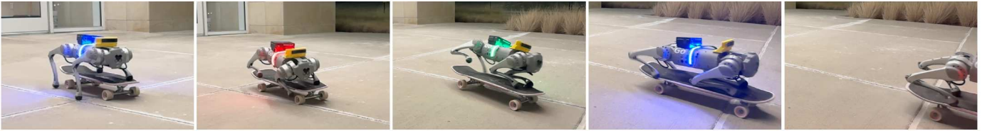
Fig. 2: The potholes on the downhill slope caused the robot dog’s right front leg to get stuck, preventing it from smoothly getting onto the board. Both of its hind legs even lost contact with the board. Nevertheless, the policy could still guide the robot dog to jump back onto the board and complete the recovery behavior.
