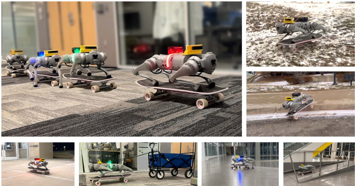
Fig. 1: Demonstration of DHAL performance across various indoor and outdoor terrains, including slopes, carpets, sidewalks, step, and scenarios with additional payloads or disturbance. The controller enables the robot to perform smooth and natural skateboarding motions, with reliable mode identification and transitions under disturbances.
